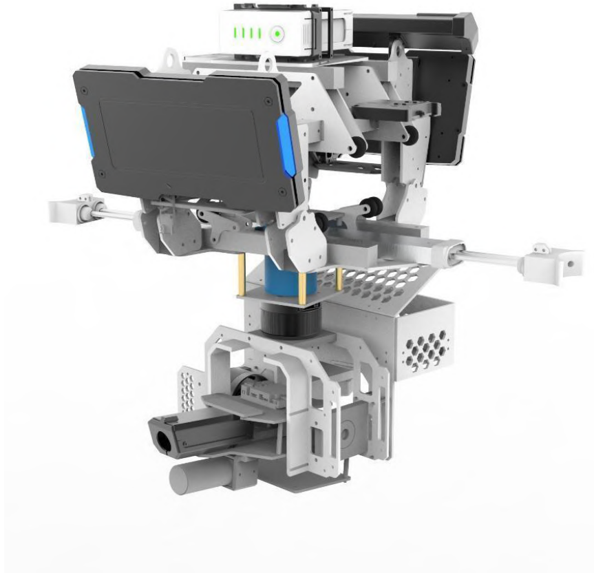
Figure 4. A photo of the 2021 Sentry robot, which shoots 17 mm projectiles and serves as the guardian of the base. This year, the Sentry robot will be terrestrial.
